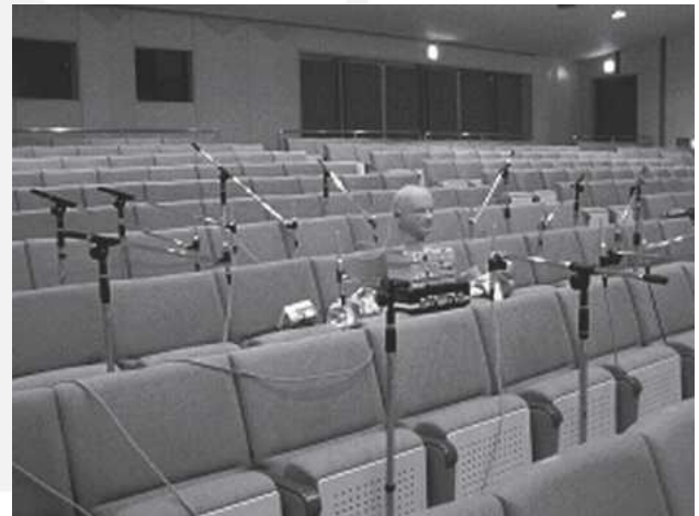
Fig. 8. Side view of microphone arrangement.
